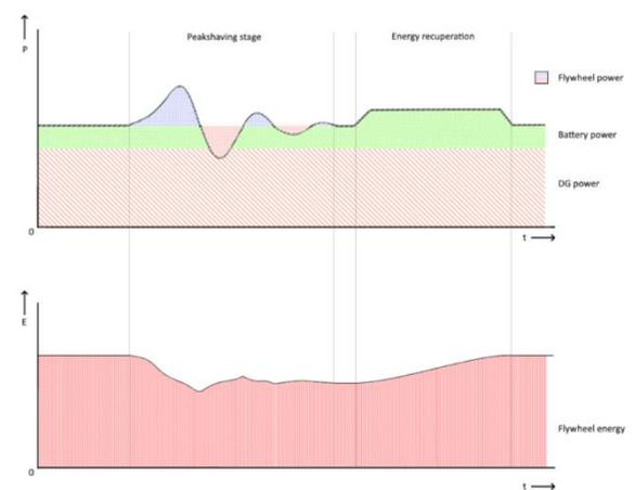
Figure 11: Flywheel behaviour on a hybrid cutter system
