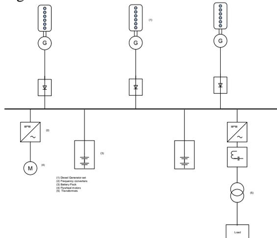
Figure 9: Hybrid cutter system with a flywheel
