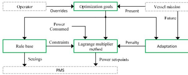
Figure 2: Energy Management System architecture
