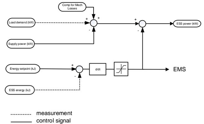
Figure 10: Flywheel control system architecture
