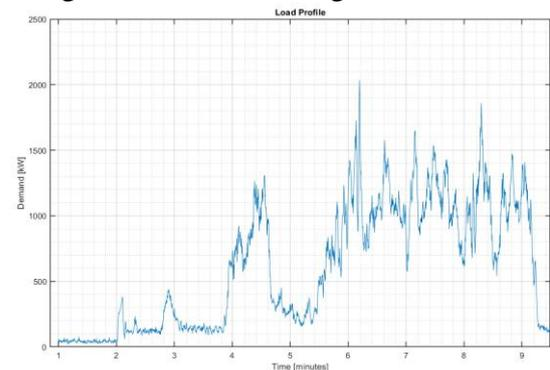
Figure 8: Load profile of a cutter suction dredger
