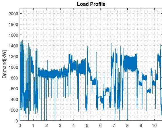
Figure 6: Load profile of the hybrid super yacht
